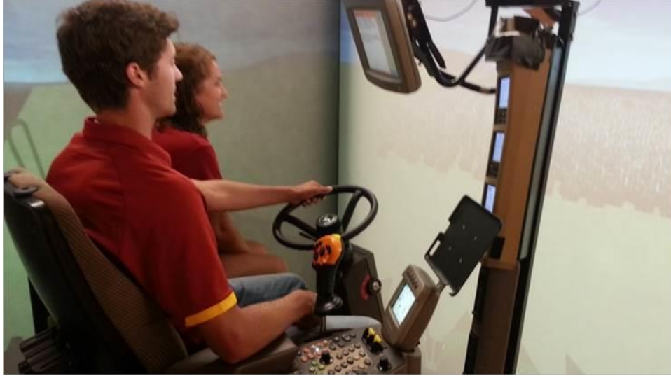
Figure 4. Operator driving the combine simulator with a research team member riding in the buddy seat.
