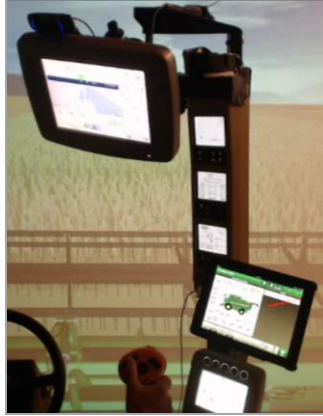
Figure 1. Harvest information displayed on four primary displays; from top down the navigation display, corner post display (3 small screens), the iPad with novel harvest technology, and the command arm display (bottom).
